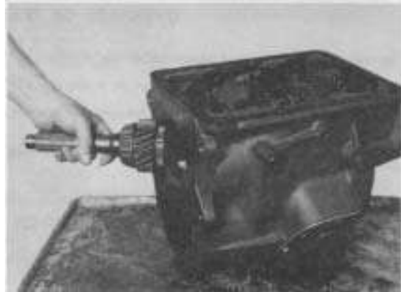
Figure 8 - Remove main drive gear and bearing assembly.
