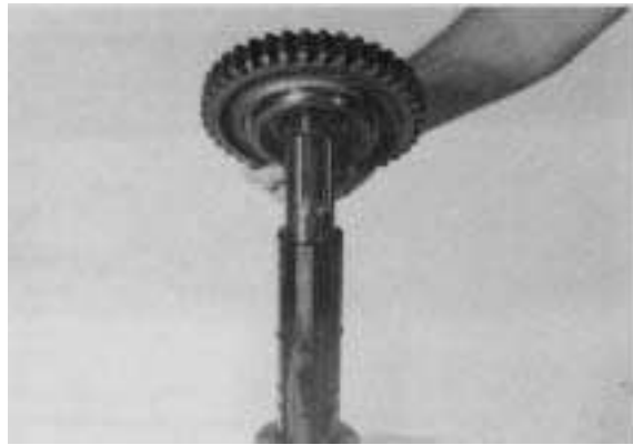
Figure 33 - Remove 1st & Reverse sliding gear.
