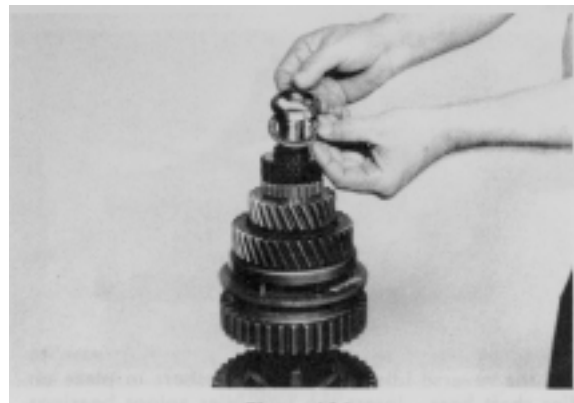
Figure 106 - Position 4th & 5th shift hub bearing and bearing race on mainshaft.
