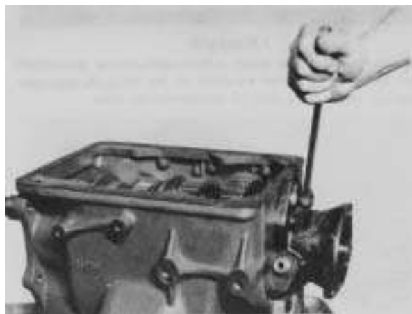
Figure 3 - Lock transmission in two gears and remove brake drum or universal joint nut. Remove mainshaft rear bearing cap bolts and washers and stud nuts and washers.
