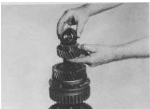
Figure 24 - Remove shift hub sleeve and 4th gear.
