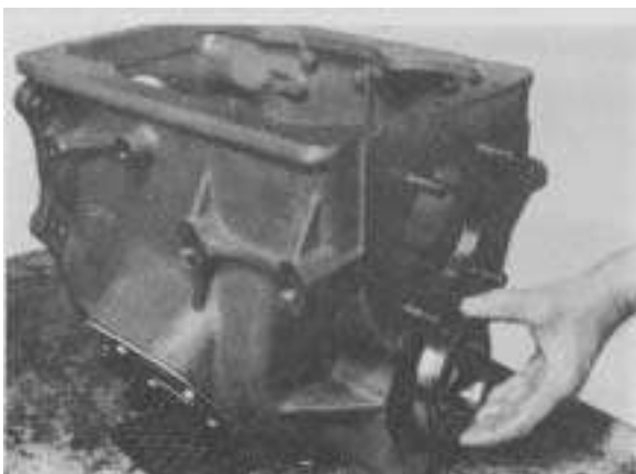
Figure 18 - Tap countershaft rear bearing out race from case.
