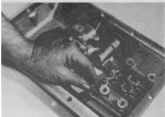
Figure 47 - Remove mesh lock poppet balls, quantity 4.
