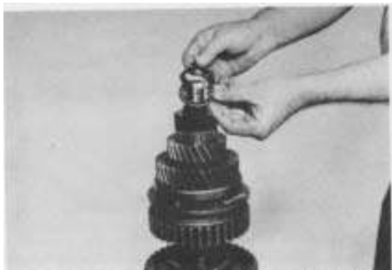
Figure 23 - Remove shift hub bearing race and bearing.
