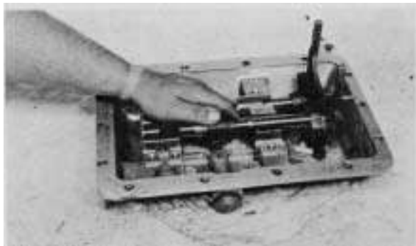
Figure 89 - Install 1st & Reverse shift lug, rocker lug, shift rail and spacers in rail groove over mesh lock balls and spring. NOTE: Position widest spacer between shift lug and front support. The narrower spacer between the shift lug and center support.
