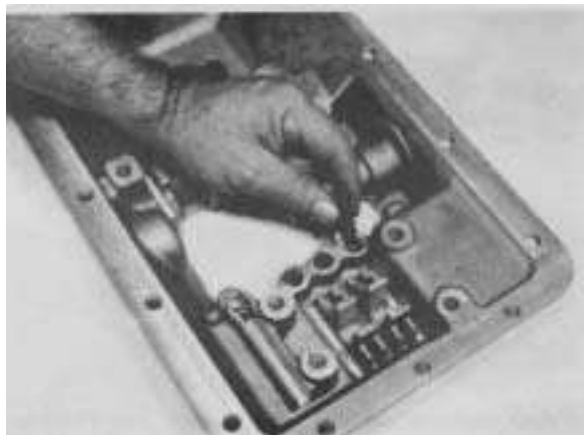
Figure 55 - Install poppet springs, quantity 4.
