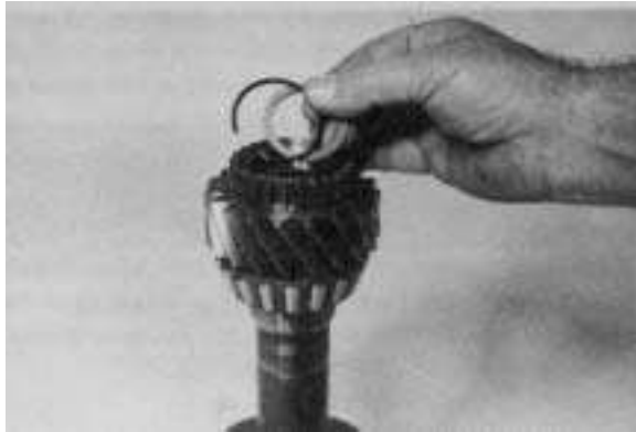
Figure 95 - Install roller bearing washer and retainer ring.
