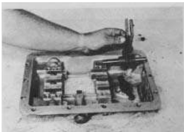
Figure 79 - Remove 1st & Reverse shift fork and rail assembly.
