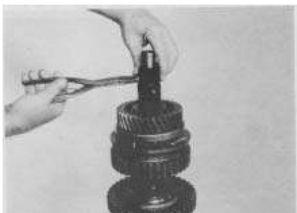
Figure 25 - Remove 3rd gear retaining ring.
