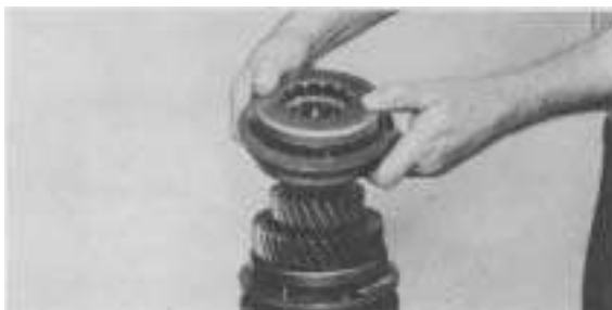
Figure 22 - Remove 4th & 5th synchronizer and synchronizer cups from mainshaft.
