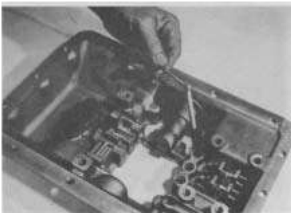
Figure 48 - Remove poppet springs, quantity 4.
