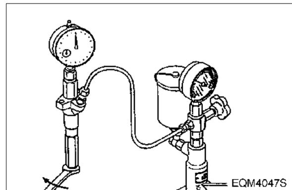
i. Operate the nozzle tester and increase the tester pressure up to 350 ~ 450 kgf/cm<sup>2</sup> in order that the needle valve can be fully lifted. Then, record the full lift value "L".
