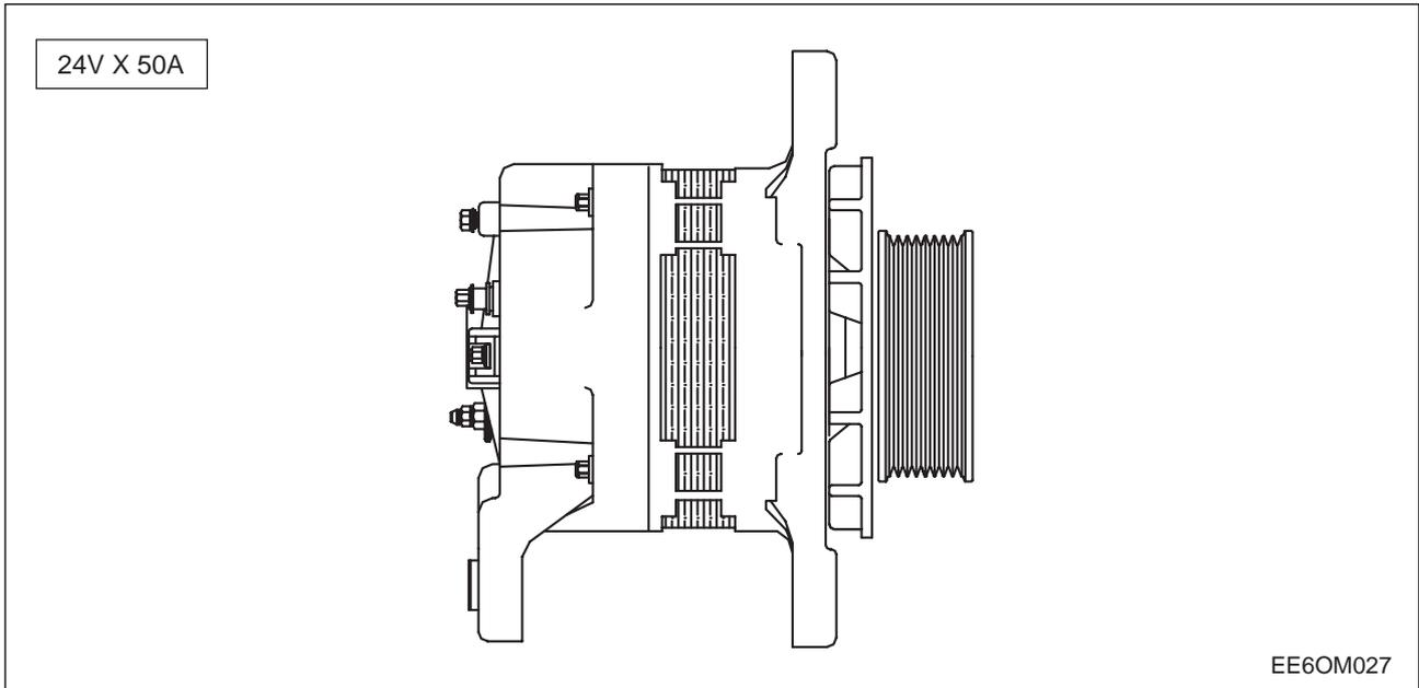
The alternator is maintenance-free, nevertheless, it must be protected against dust and, above all, against moisture and water.
