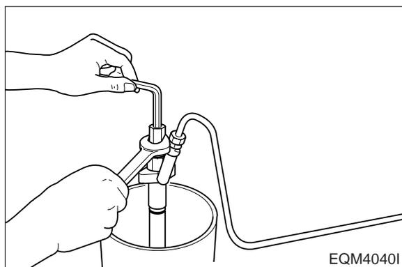
n. With a monkey wrench, fix the nozzle holder securely and tighten the cap nut (SW 19mm) to specified torque.
