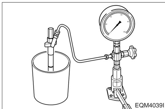
m. Adjust the primary opening pressure to the specified pressure using the adjusting screw (4).
