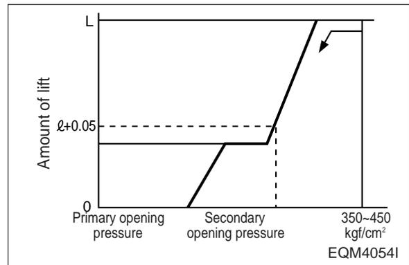
c. Take the indicated value on the pressure gauge at the point of time when the needle of the dial gauge indicates the specified needle valve lift value. (In general, pre-lift “  $l$  ” + 0.05mm. Refer to following figure.)
