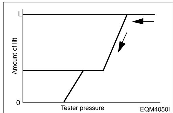
b. Take the indicated value on the dial gauge at the point of time when the secondary spring completes its operation and the needle valve puts an end to descent (the position of needle valve lift value “  $l$  ” as shown in the above and right figures) and check that the value is within the specified limit.
