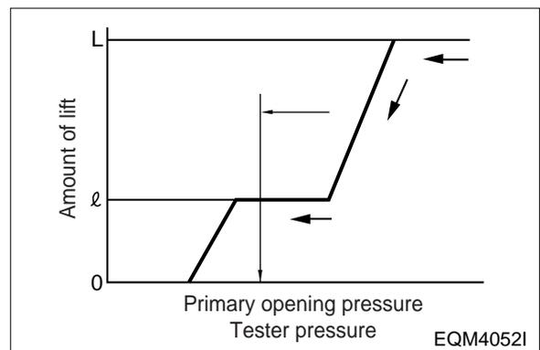
c. If the measured pre-lift value deviates from the specified limit, replace the pin (14, 16), lift piece (13), spacer (15), and nozzle assembly (A) with a new “nozzle service kit”.
