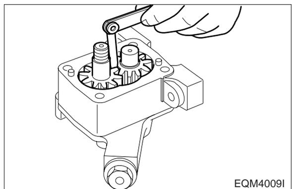
(3) Measuring clearance between drive shaft and bushing
