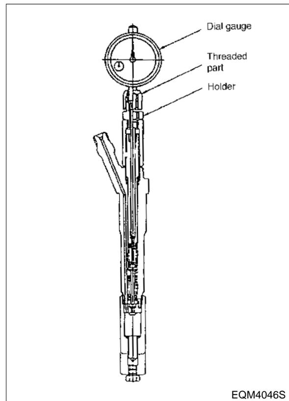
g. Assemble the nozzle and nozzle holder assembly to the nozzle tester and zero the dial gauge.
