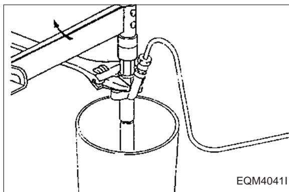
■ **Inspecting the needle valve for full lift**
