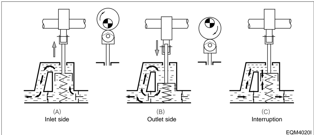
The fuel pressurized as the cam rotates on flows through the check valve on the outlet side as shown in (B). If the feeding pressure increases abnormally, the spring is compressed, resulting in interrupting further delivery of fuel as shown in (C).
