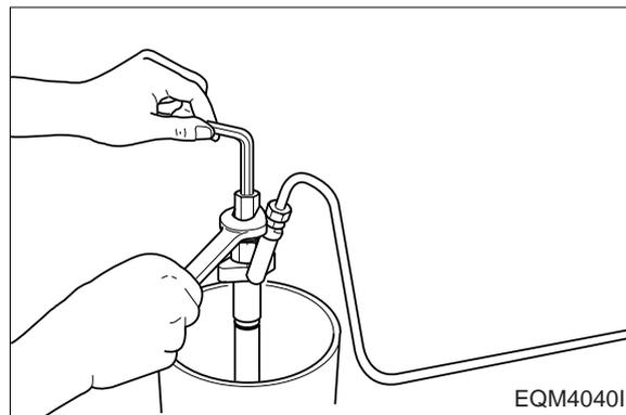
b. If the secondary opening pressure still deviates from the specified limit in spite of the readjusting the primary opening pressure, take off the nozzle fixing portion from the nozzle holder and remove the adjusting shim (10).
