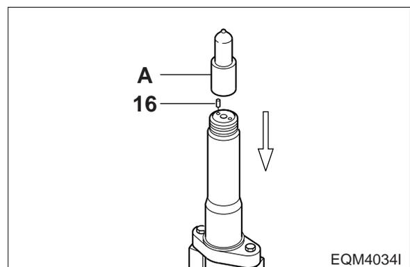
g. After installing the gasket (157892-1500) on the nozzle, use the cap nut (157892-4000 : SW22mm) to fix the nozzle onto the nozzle holder.
