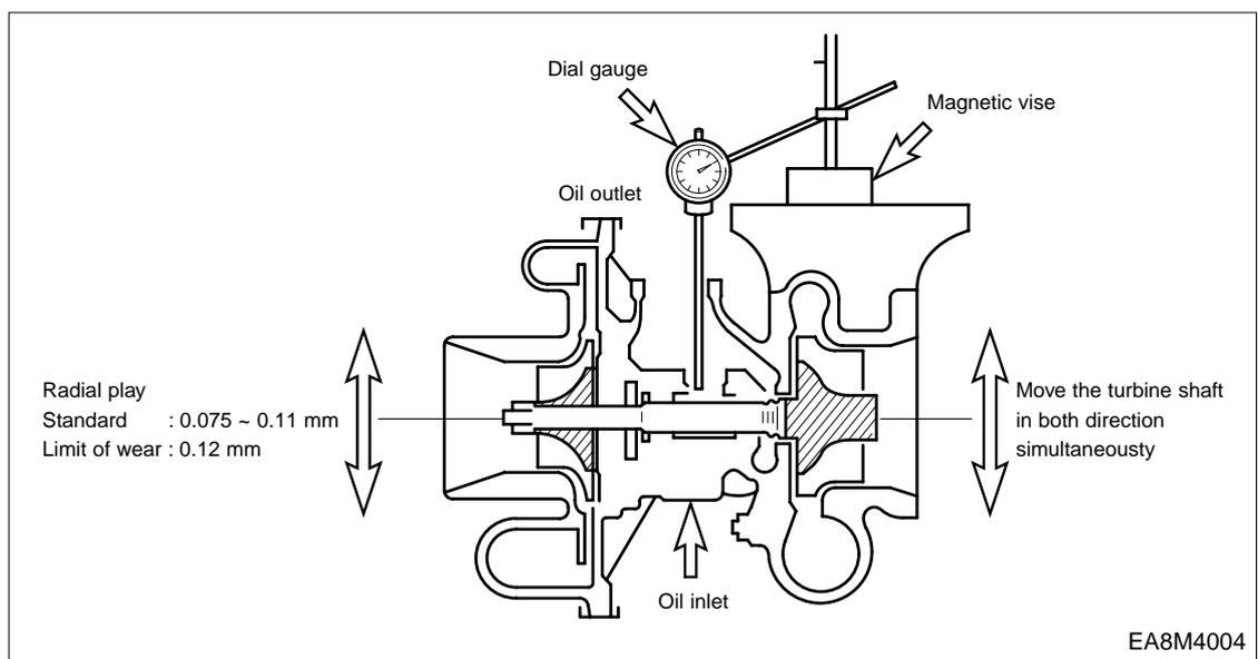
(3) If the measured axial and radial plays are beyond the limit of wear, replace or repair the turbocharger.
