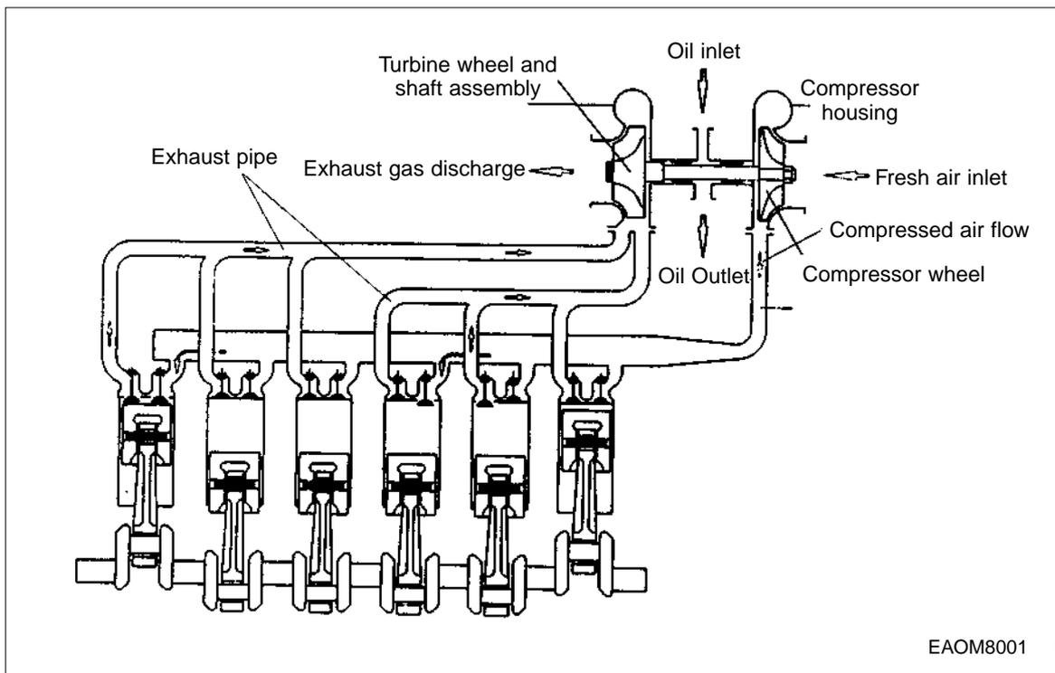
The turbocharger is a system designed to make use of the engine exhaust gas energy to charge high-density air into the cylinders, thereby to increase the engine output.
