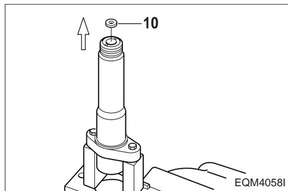
d. After replacing the existing adjusting shim, measure the secondary opening pressure and continue the adjustment until a value satisfying the standard value.
