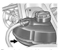
The coolant surge tank is near the center of the engine compartment. See *Engine Compartment Overview* on page 10-3 for location.
