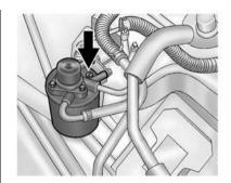
Locate the fuel filter vent valve on top of the fuel filter housing. Turn the valve screw counterclockwise several full turns to open.
