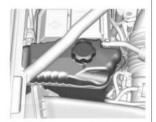
The coolant surge tank is in the engine compartment on the passenger side of the vehicle. See Engine Compartment Overview on page 10-3 for location.
