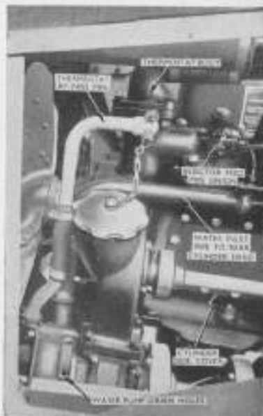
Fig. 17. Part View—Nearside Front of Engine.
